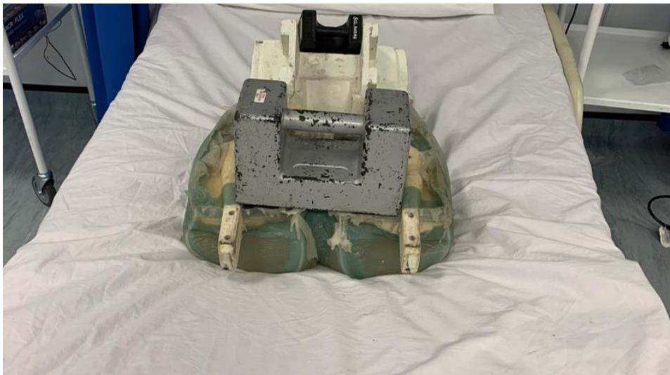
Figure B-1: A static test involving loading of a buttock model with an additional weight of 22.5 kg onto a foam mattress incorporating the ForeSite PT pressure mat.
