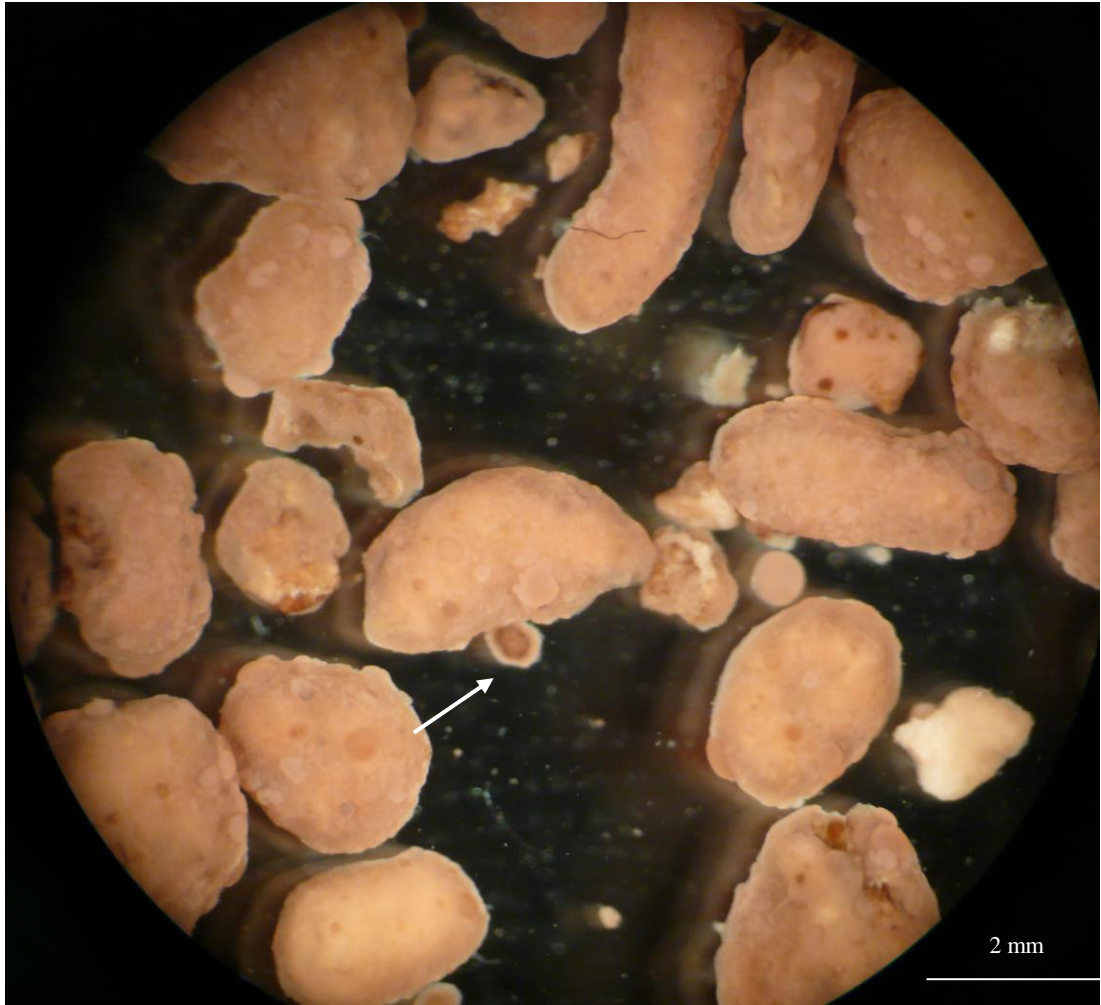
Figure 3.20 - Mixture of different sizes granules before characterisation study. The arrow indicates a bud.
