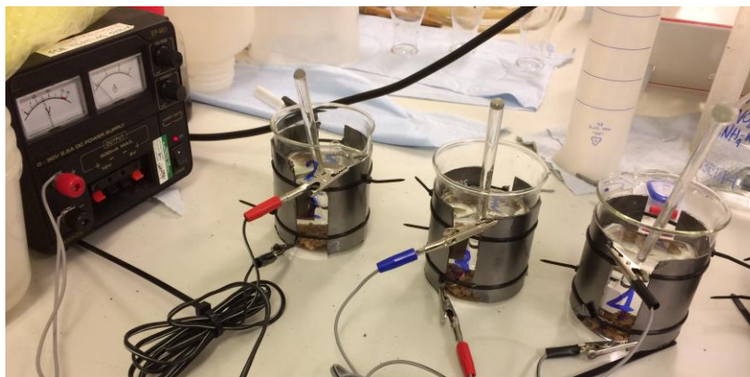
Figure 5.1 – Electric field setup showing power supplier and the samples containing beaker.
