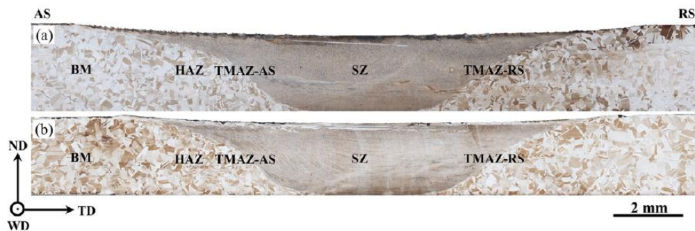
Figure 2.3 Low magnification optical micrograph of friction-stir welded super-austenitic stainless steel S32654 joint manufactured at different rotational speeds: (a) 300 rpm and (b) 400 rpm [37]
