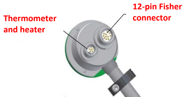
Figure 3.39 The original connection panel layout with all singles mixed in one 12-pin Fischer connector[134].
