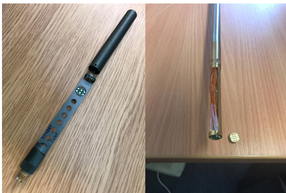
Figure 3.41 (Left) The original chip carrier mounted tube, which could mount 2 chip carriers at the same time. (Right) The re-designed chip carrier mounted tube, which only had 2 chip carrier position, but low noise level.
