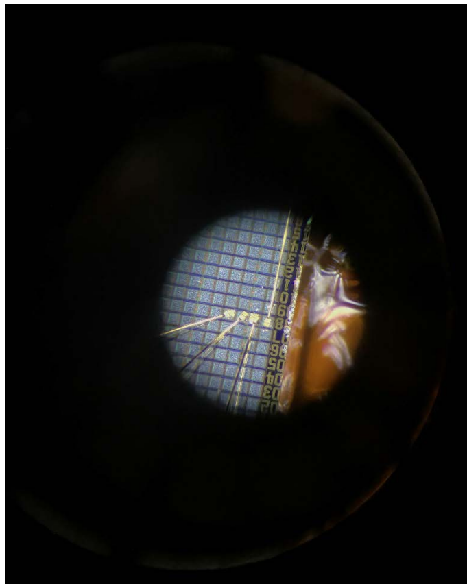
Figure 3.12 The MOSFETs samples mounted to a 6-pin chip carrier with a yellow no-conductive epoxy.
