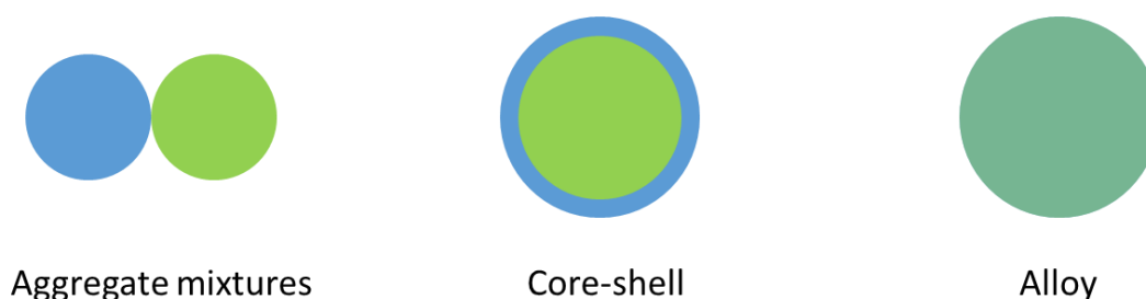
Figure 1-2 Schematic illustration of the three main mixing patterns of bimetallic nanoparticles ( A_mB_n ).
