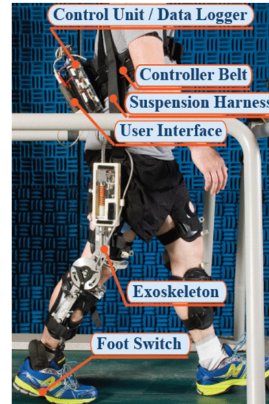
Figure 2.6: The quasi passive knee system from Shamaei et al. (2014)
