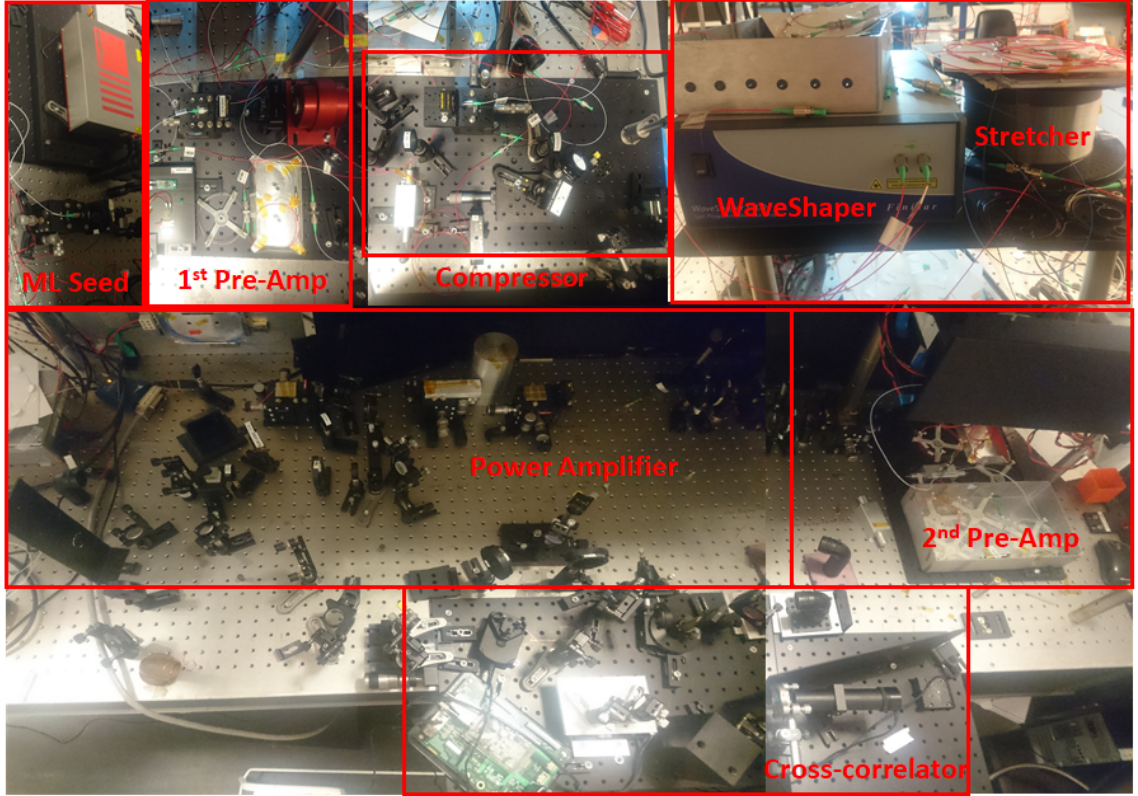
Figure 7.10: Full laser system image including the mode-locked (ML) seed, NKT laser.
