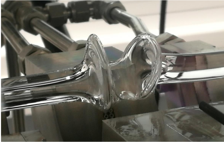
Image 17. TDF pedestal structure fail fabrication
