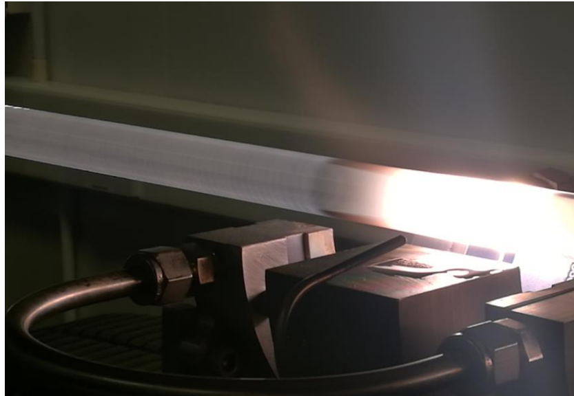
Image 16. Fully sintered aluminosilicate layers for pedestal structure
