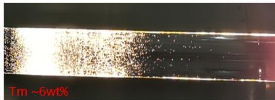
Image 15. HGSD-02 preform after sintering (Tm ~6wt%)
