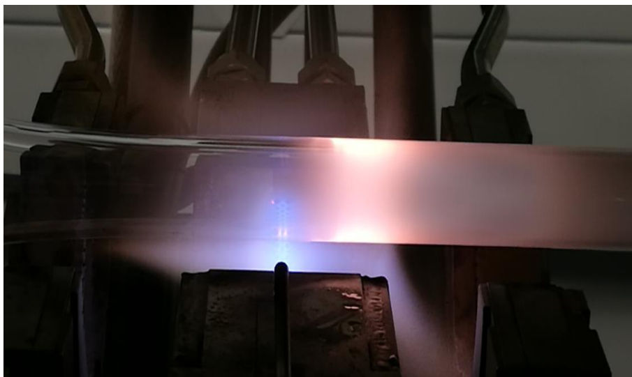
Image 2. MCVD process during \text{SiCl}_4 and \text{AlCl}_3 deposition (core formation)
