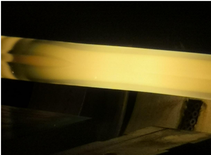
Image 24. LMA Yb-doped preform during collapse stage
