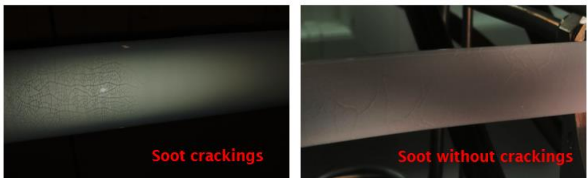
Image 20. Enhanced porous soot layer after solution doping
