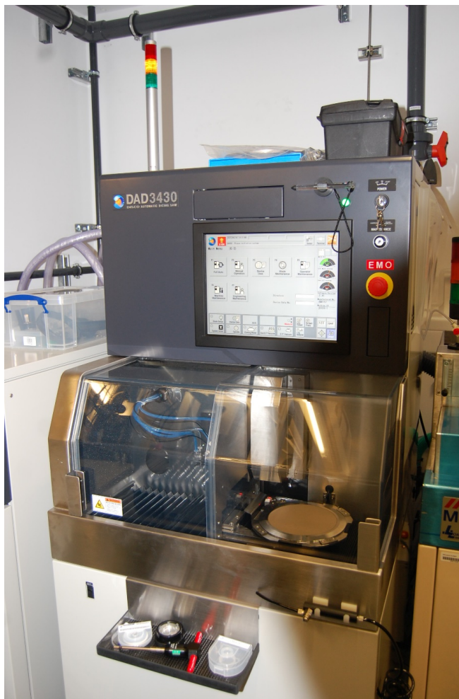
FIGURE 4.3: Photograph of the dicing machine used for the fabrication of the zinc-indiffused PPLN ridge waveguides presented in this thesis. Photo courtesy of Dr. Lewis Carpenter.
