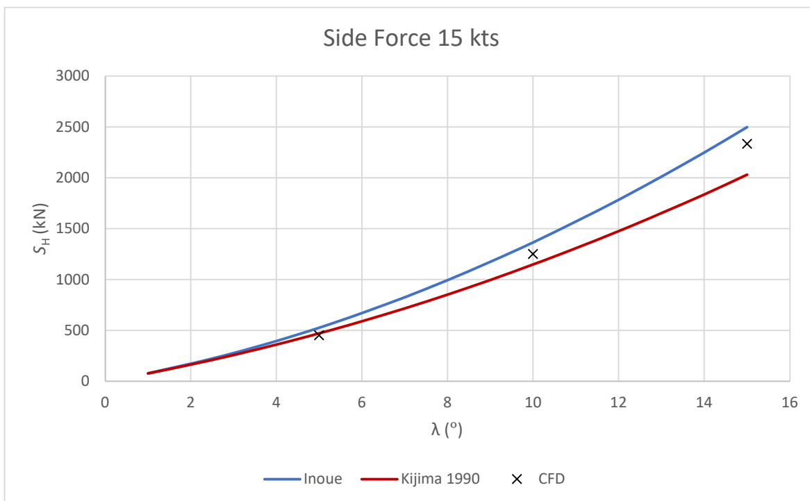
Figure 118: Comparison of S_H from CFD with estimated S_H for Storm Cloud at V_s = 15 kn
