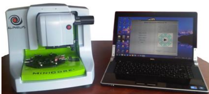
Figure 24. Tissue Arrayer Minicore®3 (ALPHELYS, France) for TMA creation
