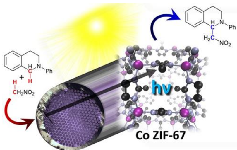
Figure 1. Schematic showing our unique methodology for creating an all-inclusive photocatalytic microreactor, coating a metal organic framework (Co ZIF-67) within the channels of an optical fibre, and potential applications for C-H activation to selectively form C-C bonds.
