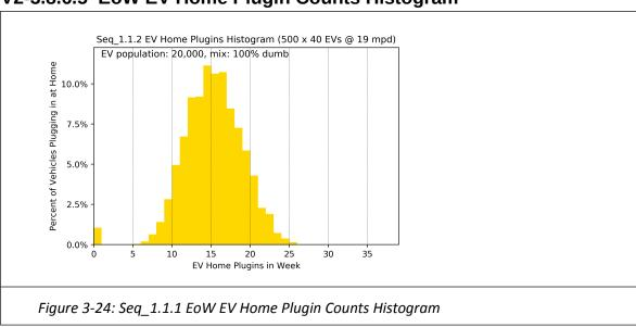
Home plugin frequency is surprisingly high. This was found driven by reduction of the EV battery capacity due to low ambient temperature. In winter, when EV loads are higher, the battery can store less hence EVs are plugged in more often. This is a learning point:
