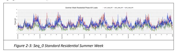
Summer Week Residential Loads are for the hottest week in 2013 (from 15th July 2013). Note kW scale is 0-35 kW vs. 0-60 kW. It is unlikely that AC was in use. Phase 2 (green) is consistently low.
