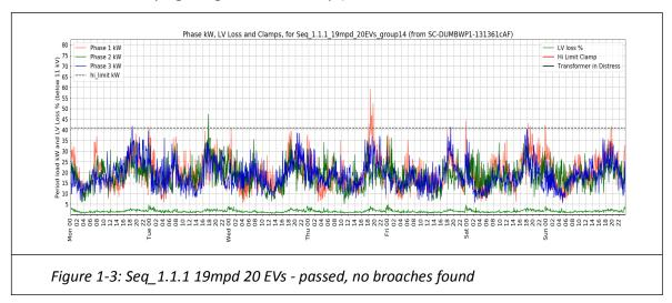
To the eye this is near identical to the baseline feeder load. Next is a "fail" plot:
