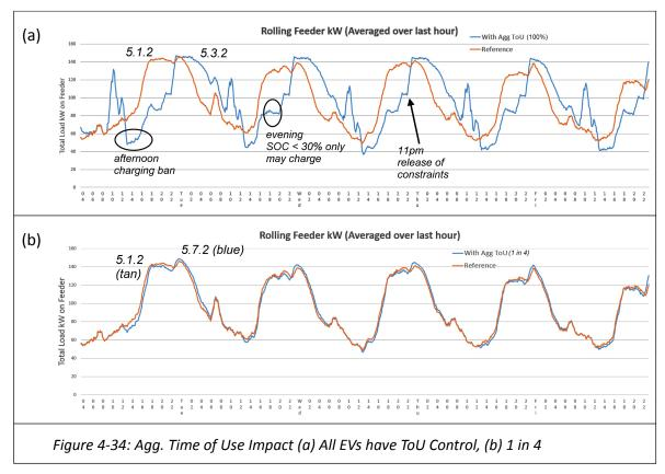
In (a), Aggregator control gives a clear effect - deferring a charging peak, plus causing significant EV disruption. Yet for (b), with 1 in 4 EVs under Aggregator control, there is negligible network load effect, plus the method provokes EV undercharging.
