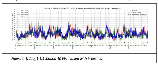
Why does Figure 1-3 not blow, given the peaks exceed the hi\_limit line? Peaks were insufficient to trigger a cable fuse and infrequent enough to not exceed 2 periods at x1.5 transformer rating. Figure 1-4 failed with too many modest overloads.
