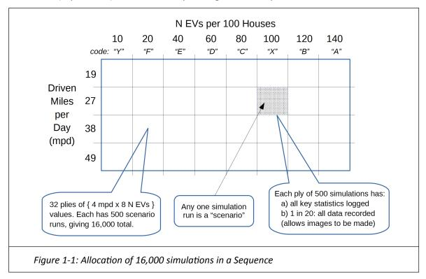
Simulations execute in batches of N EV value i.e. **columns** e.g. for 80 EVs: 500 simulated weeks at 19 mpd, repeated for 27 mpd, 38 mpd and 47 mpd. Each column takes c. 8 hours to execute but can be parallelised; the whole Sequence taking c. 1 day to run.
