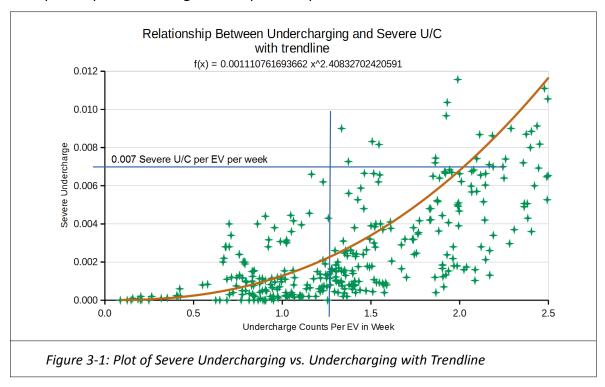
Rather than use the trendline (brown curve), we wish to avoid severe undercharging rates likely to exceed the "50:50 chance in 10 winters" level, established as 0.007 severe undercharges per EV per week. The vertical blue line, placed by eye, marks a plausible partition with instances on the right exceeding 0.007 severe undercharges. The cross-over so found is at c. 1.25 undercharges per EV per week.
