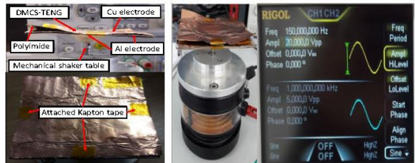
Fig. 4. Fabricated DMCS-TENG mounted on the mechanical vibrator for the output performance measurements.
