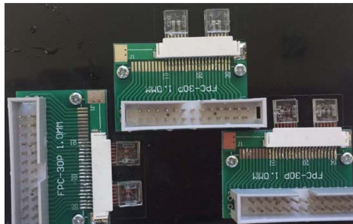
Figure 7-11: A photo of a customized detection board. The detection board contains six impedance detection chips and three customized PCB holders. Each PCB holder was used to transmit signals for two impedance detection chips.
