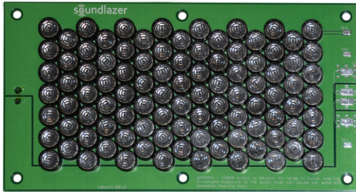
FIGURE 3.6: Example of a parametric array loudspeaker, consisting of numerous ultrasonic transducers. Picture as displayed in (Haberkm, 2020).
