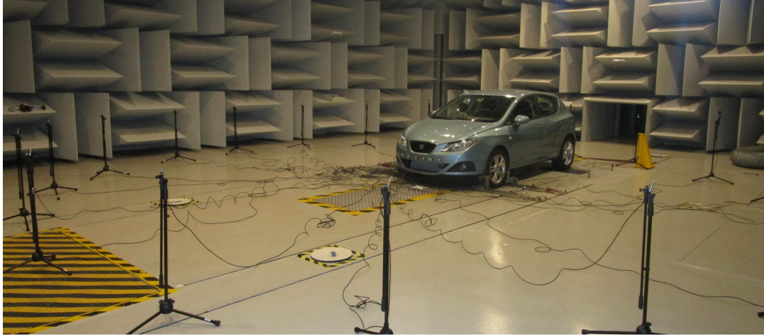
FIGURE 6.1: Test vehicle and measurement set-up in the semianechoic chamber.
