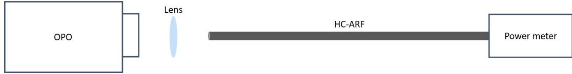
FIGURE 8.9: Cut-back measurement setup using an OPO.
