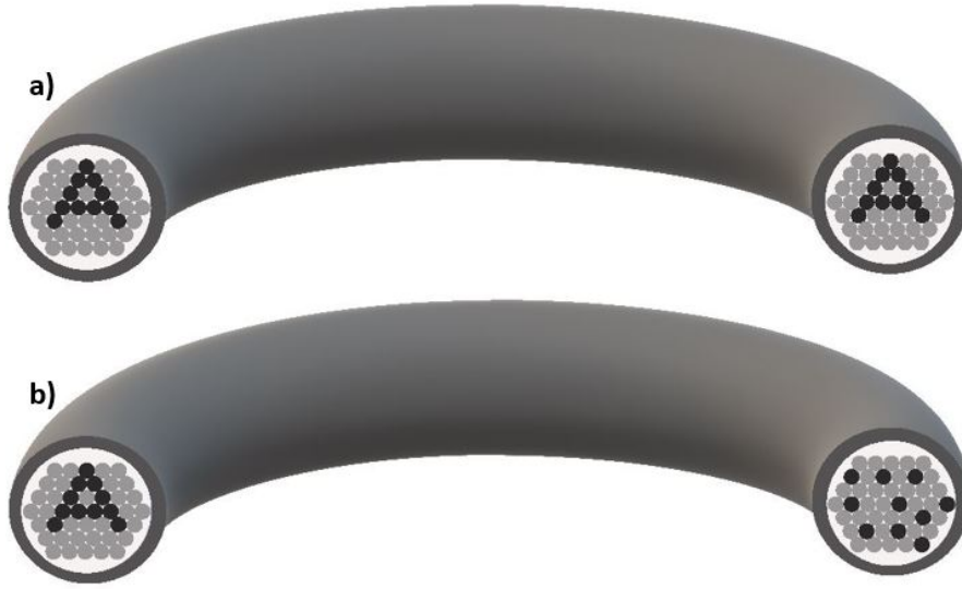
FIGURE 2.8: a) Coherent and b) incoherent fibre bundle [60].
