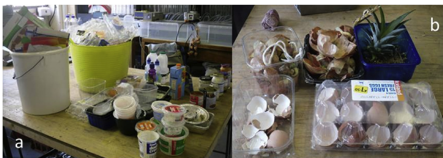
Fig. 1. Items rejected during SFW preparation: (a) Packaging materials, (b) Materials not put through macerator.
