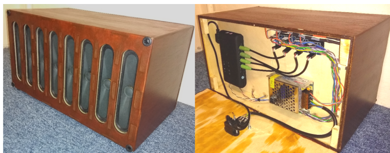
FIGURE C.1: 8-Channel loudspeaker array prototype. Left: Front view; Right: Rear view with back panel removed.
