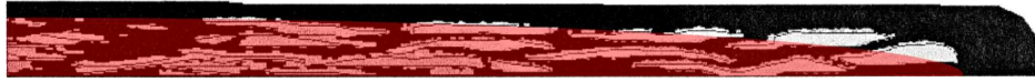
(a) Quarter-tape cross-section, Amemiya et al [73] ©1998 Elsevier. The width of the displayed quarter of the tape is 1.75 mm and the thickness is 0.125 mm, details in Table 5.1.
