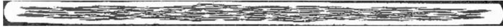
Figure 2.2: First generation multifilamentary conductor, produced from Bi-2223 superconducting material (dark filaments) and filled with Ag or similar [23] © 2004 IEEE.
