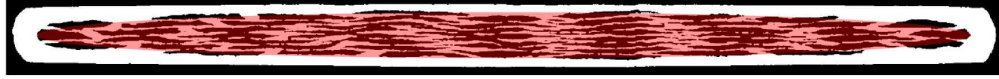
(b) Full tape cross-section, Choi et al [68] © 2004 IEEE. The width of the displayed full tape is 3.1 mm and the thickness is 0.17 mm, details in Table 5.3.
