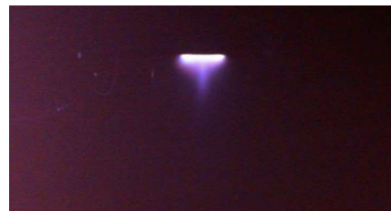
Figure 7: The MaSHEKT-100 operating within the large vacuum chamber at approximately 280 W with 6.0 sccm of krypton.
