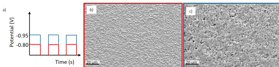
FIGURE 6.4: Schematic and SEM images of Sb_2Te_3 electrodeposited from 1.75 mM [N^nBu_4][SbCl_4] , 3 mM [N^nBu_4]_2[TeCl_6] in CH_2Cl_2 solution containing 0.1 M [N^nBu_4]Cl supporting electrolyte CH_2Cl_2 by pulsed electrodeposition ( t_{on}=5s , t_{off}=10s ) at: -0.80 (b) and -0.95 (c) V vs. Ag/AgCl.
