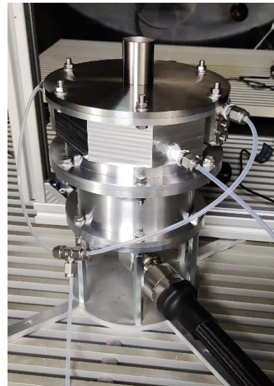
Figure 6. Mid-plane XMET with coaxial line, propellant feed and pressure tap lines attached, mounted in the vacuum chamber for testing.
