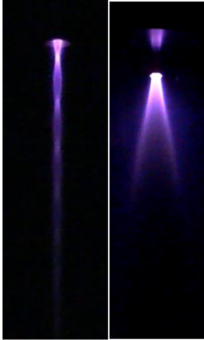
Figure 13. XMET plasma plume exiting the nozzle under rough (left) and high vacuum (right).
