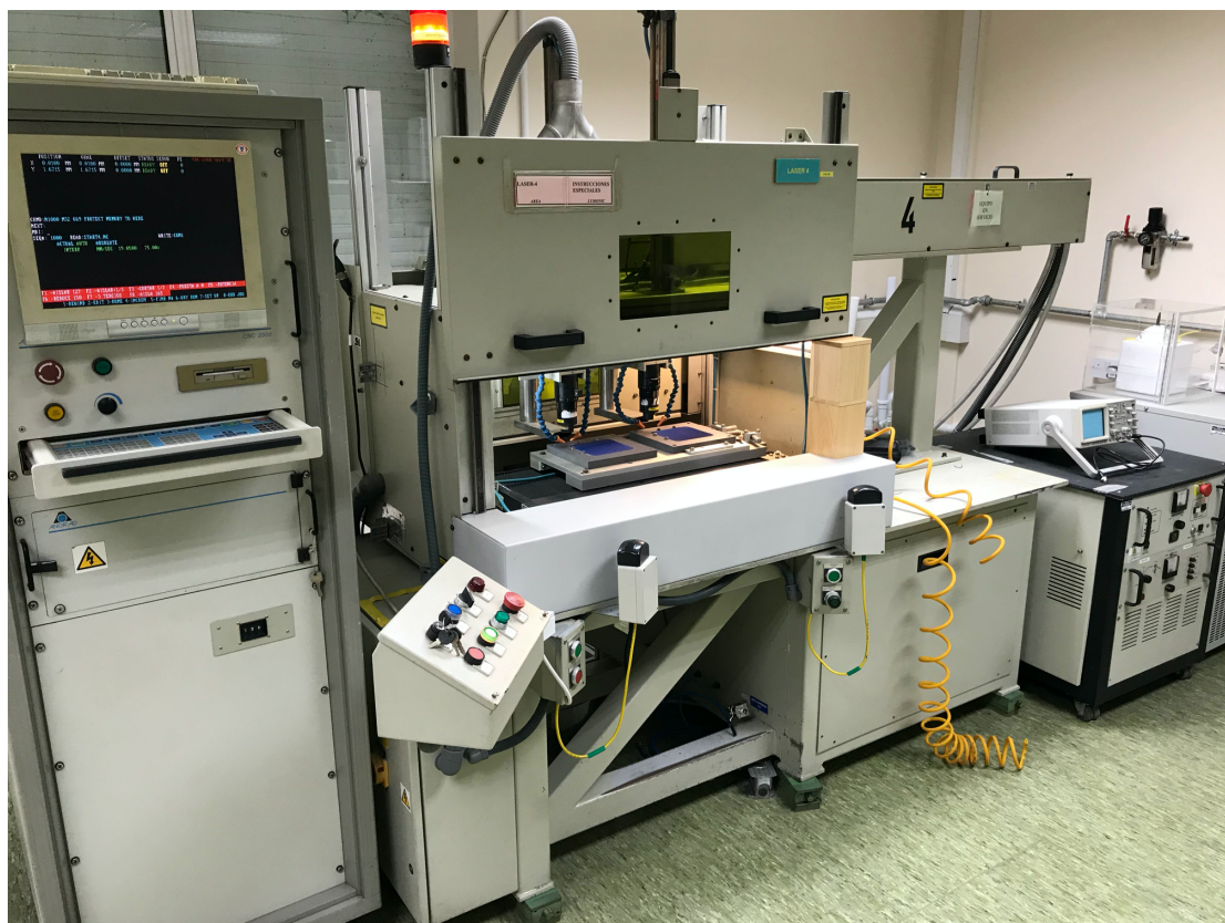
Figure 3.6 - Lee Laser Inc. 1064nm Nd: YAG laser used for Saturn cell fabrication
