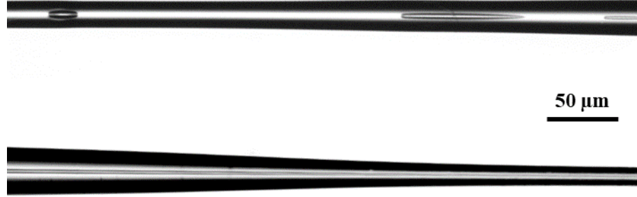
Figure 3.11 Microscope image showing SCF with core breakup (top) and SCF with continuous core (bottom).
