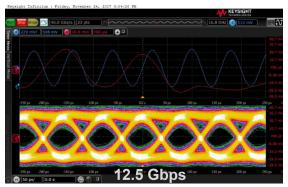
(b) NTU micro ring modulator in carrier depletion. Data rate 12.5 Gbit/s at 1973.2 nm.  $V_{bias} = -3 \text{ V}, V_{p-p} = 6.0 \text{ V}.$
