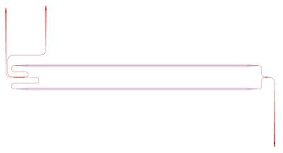
(c) Loss analysis structure will bare passive MZI.
