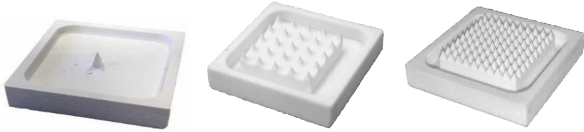
(a) A single tip emitter with 20 degrees side surface angle. (b) A P4 grade emitter with 25 two-millimetre tall tips. (c) A P5 grade emitter with 100 two-millimetre tall tips.
