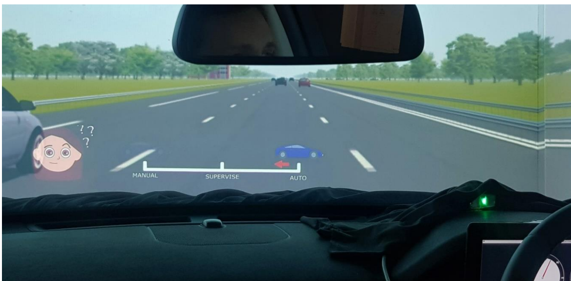
Figure 9.6. Example of an HUD slide in vehicle, augmented into the driving scenario. Slide shows Steeri prompting driver to ask her questions.
