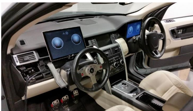
Figure 5.2 Driving simulator set-up to simulate handover between two drivers
