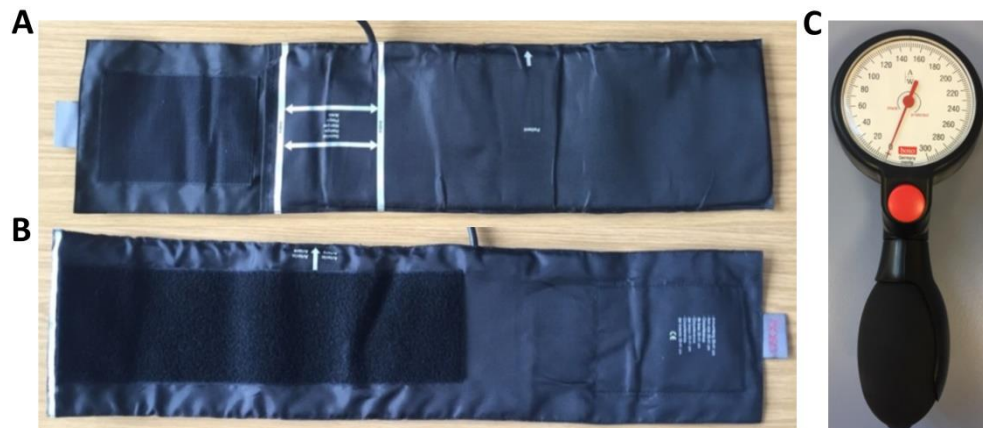
Figure 3.1 Images of A: Inner and B: Outer surfaces of BOSO Sphygmomanometer selected to load calf tissues, C: BOSO Profitest Sphygmomanometer pump and gauge
