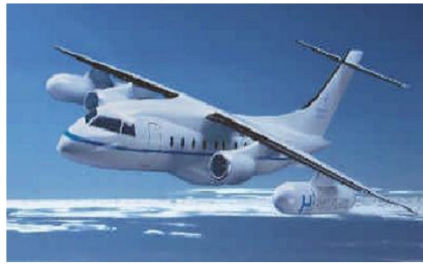
FIGURE 1.1: Hydrogen powered aeroplane with non-integral tank (source: [105])
