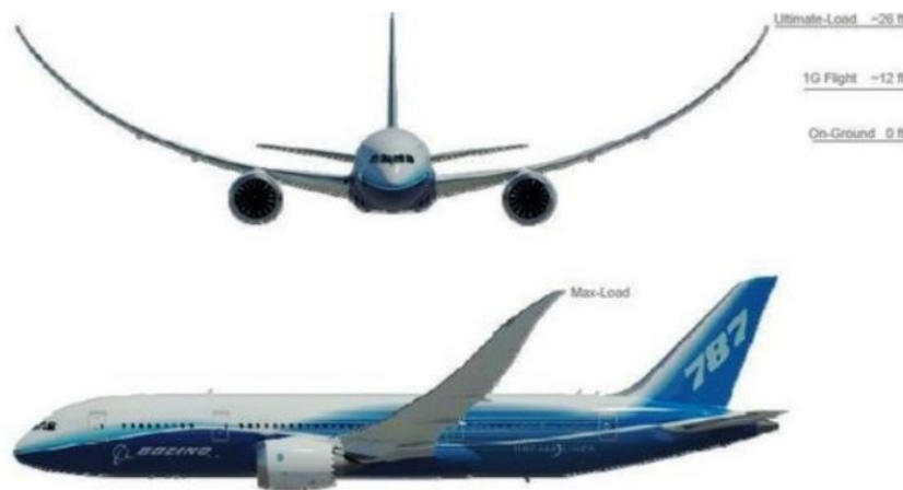
FIGURE 1.7: Wing deflection under the ultimate load of the Boeing 787 Dreamliner (source: newfoxy.com )
