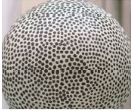
Figure 3.1: Speckle pattern applied on a sphere for DIC testing [112]
