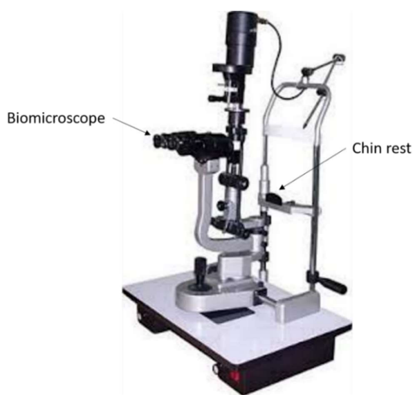
Figure 13. Slit lamp biomicroscope. The patient's head is held steady by the chin rest so the eyes can be examined by the clinician. Adjustments can be made to magnification and light intensity.
