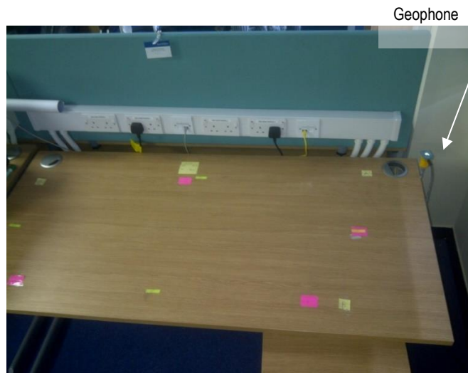
Figure 30 Desktop test set-up (1600 x 800 mm)
