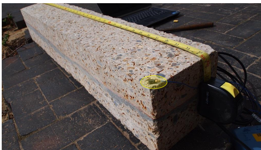
Figure 43 Test set-up - spatial decay of coherence in a particulate composite matrix with the accelerometer location highlighted in yellow
