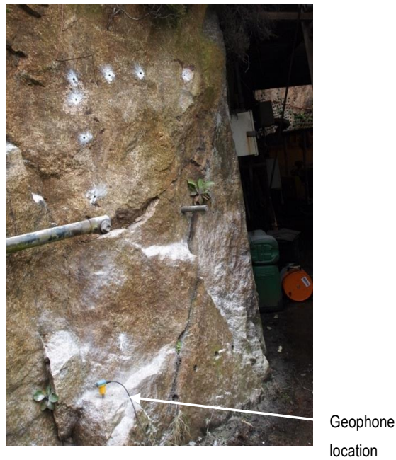
Figure 56 close up of the detonator hole arrangement with one of two positions of the geophones
