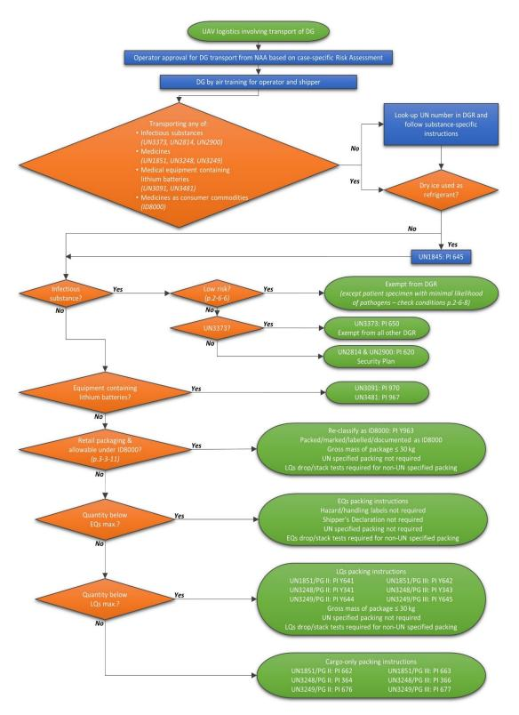
**Figure 1.** Guidance for transporting the DG likely to be involved in UAV medical logistics. Page number references relate to ICAO Doc 9284 [17].
