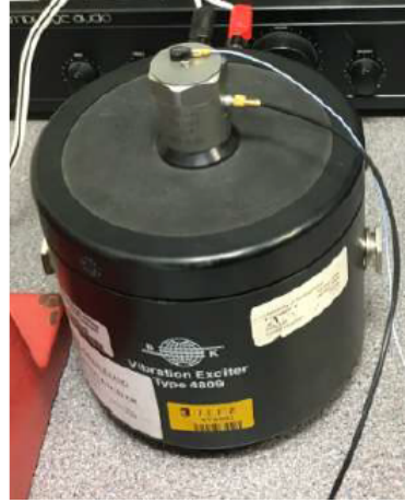
FIGURE A.1: Placing a PCB accelerometer on top of the shear accelerometer to calibrate them and check the existence of the phase lag between any two transducer.
