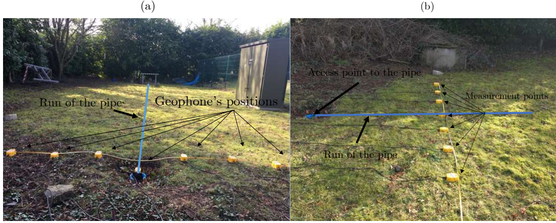
FIGURE 6.4: Experimental set up employing an in-pipe excitation technique to locate buried MDPE pipes. (a) Illustration of the third geophone array, the excitation source located on the ground surface and the pipe's main axis at the surface. (b) The position of the sixth geophone array.
