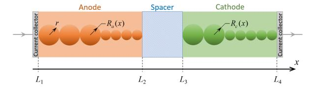
Figure 1: Schematic of a planar LIB cell. The macroscopic and microscopic coordinates, x and r, are indicated, along with the particle radii and positions between the different cell components.
