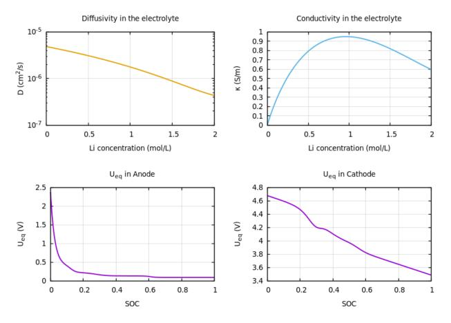
Figure 4: Ionic diffusivity (top left) and conductivity (top right) of the electrolyte, open circuit voltages of graphite-silicon anode (bottom left) and  $\text{LiNi}_{1-x-y}\text{Mn}_x\text{Co}_y\text{O}_2$  cathode (bottom right). Experimental data from from [27].
