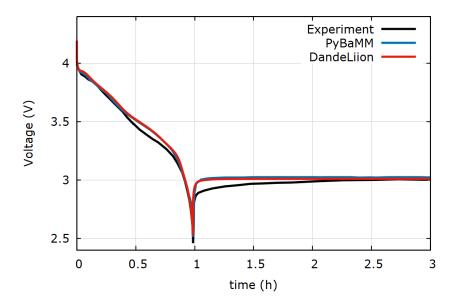
Figure 6: Cell voltage profiles computed from DandeLiion in comparison with the experimental and simulation data from [27].
