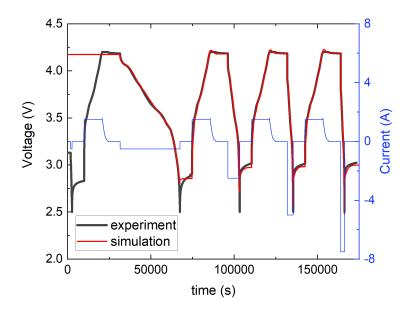
Figure 7: Cell voltage and the current vs time comparing DandeLiion simulations and experiment taken from [33]. The current varies between (dis)charge rates ranging between  $\pm 1.5$ C.
