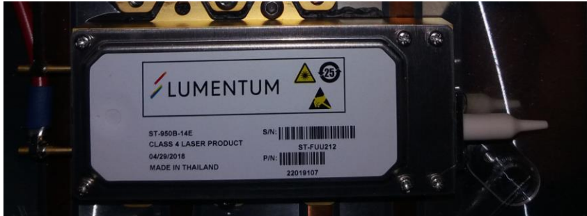
Figure 26. Lumentum ST (140W, 106µm fibre, 0.1NA)
