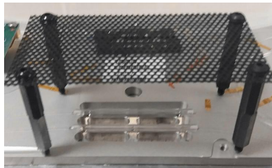
Figure 117. Cladding mode strippers surmounted by metallic grid.
