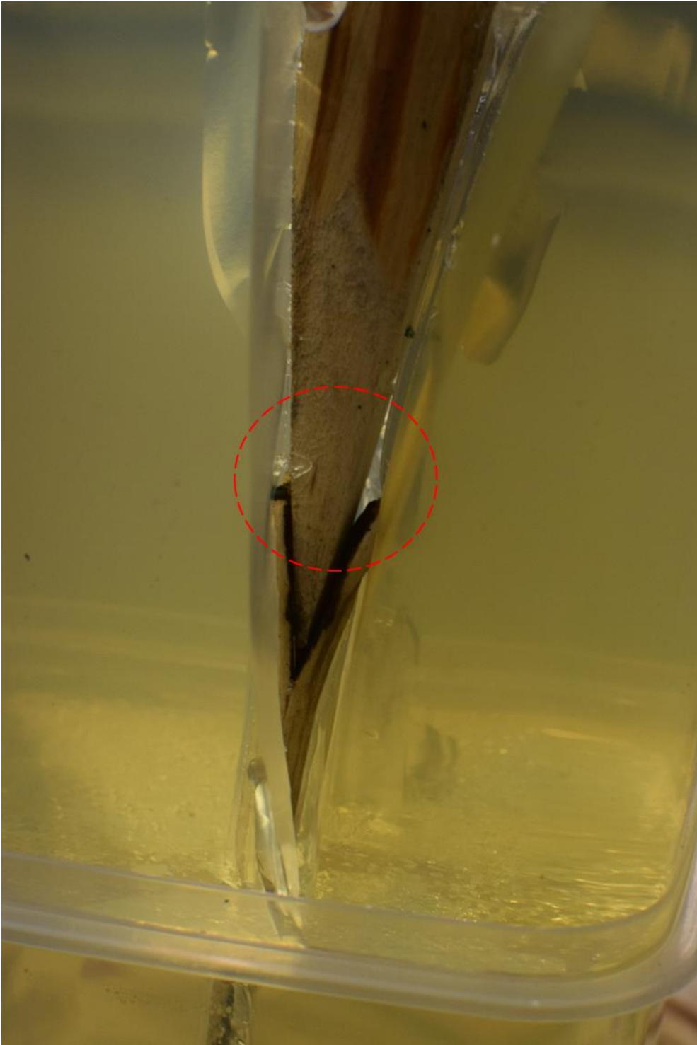
Fig. 74: Tip C series 3: before the shaft was withdrawn by the hammer, it was noticeable that although the shaft kept the wood open (though plugged), the wings of the SBP actually opened the wound wider than the shaft to a width of approximately 45mm.
