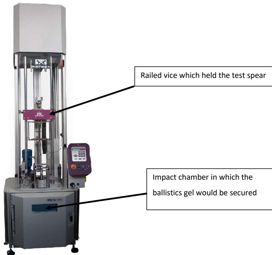
Fig 42: Instron drop tower ISO 6603. (From Instron.co.uk)
