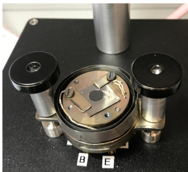
Figure 4.2.4: NAP-XPS sample holder on the B07 beamline, DLS, with a 8 mm pressed pellet of 50 mg LaMnO 3
