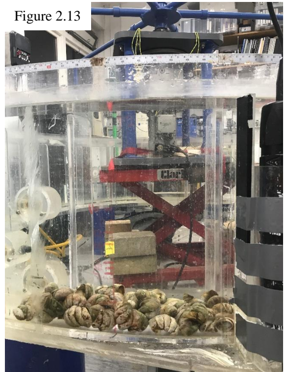
Figure 2.12 and Figure 2.13. Crepidula fornicata placed into the annular flume at a high density to create a bed structure. Plan view (Figure 2.12) and side view (Figure 2.13).
