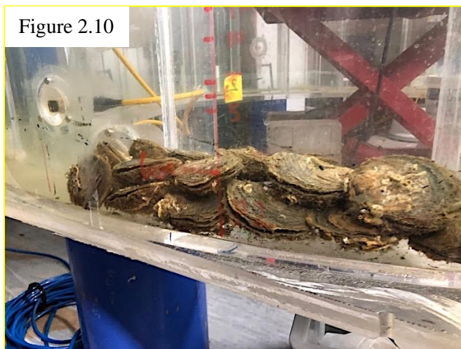
Figure 2.10 and Figure 2.11. Ostrea edulis placed into the annular flume at a high density of 367 oysters \text{m}^2 to create an oyster bed structure (Figure 2.10). ADV probe positioned to take measurement at P3 (Figure 2.11).
