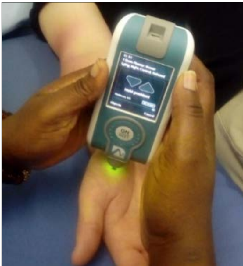
Figure 7-2: Measurement of the thenar muscle mechanical properties using the MyotonPRO device
