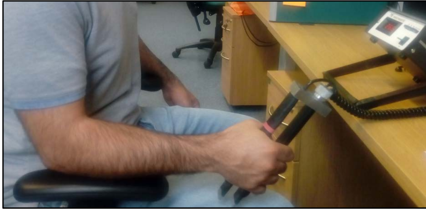
Figure 7-4: Measuring maximum hand grip strength with the MIE digital analyser
