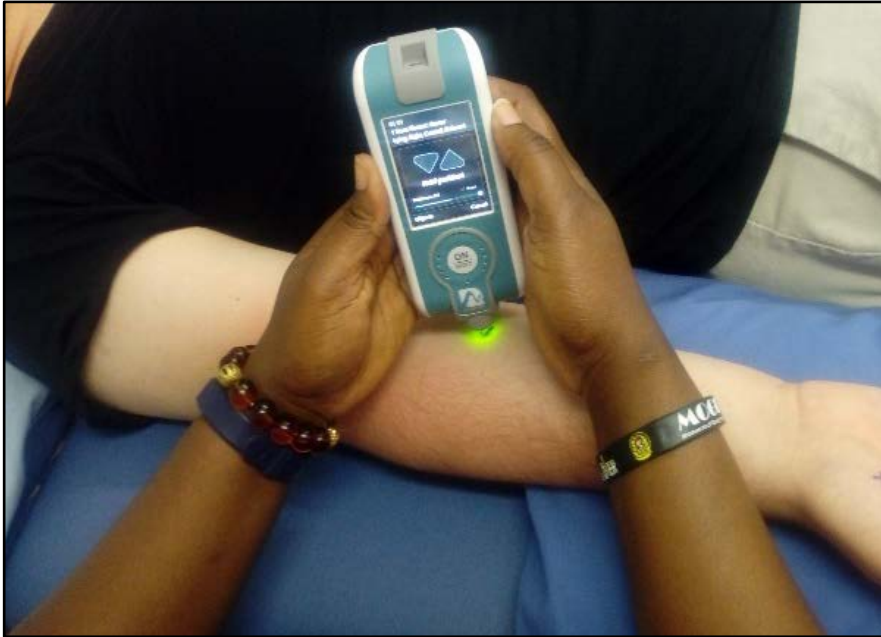
Figure 7-3: Measurement of the flexor carpi radialis muscle mechanical properties with the MyotonPRO device
