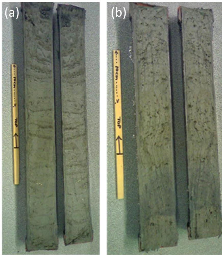
387 388 Figure 2: Photograph of the split core collected from (a) the Calshot site and (b) the Mercury 389 site showing darker silt layers (a) and residual gas voids (b). Recalling the rig lay out (Fig. 1), 390 the first, second and third hydrophones were buried at depths of approximately 21 cm, 35 cm 391 and 50 cm, respectively. The dark grey color, as well as the hydrogen-sulphide odor, of the 392 sediment core indicated that the measurements took place in the sulphate reduction zone.
