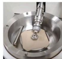
Fig. 1. Appearance of MTM tribometer (a) polymer plate specimens, (b) set-up and (c) schematic configuration.
