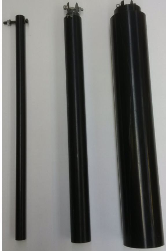
FIGURE 3.7: PVC model piers used for experiments. Left to right: 25 mm, 50 mm and 100 mm diameter.
