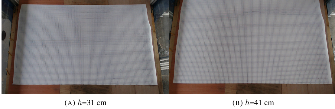
FIGURE B.1: Ruled paper used as mesh at two different water depths captured by the top camera. Mesh size 10 mm.
