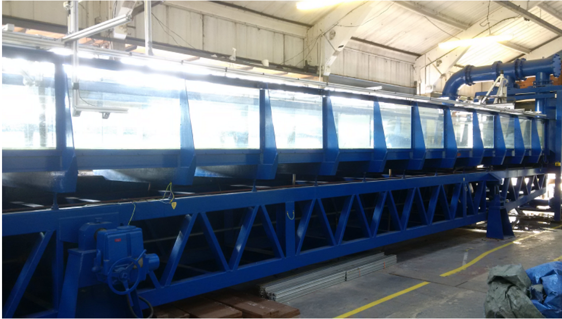
FIGURE 3.2: Side view of Chilworth internal flume at the University of Southampton Science Park.
