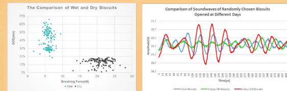
A clear difference in terms of SOS vs Breaking Force was identified for the wet and dry biscuits.
