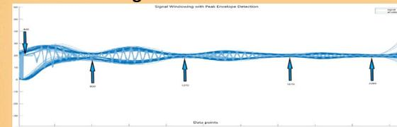
The speed of sound (SOS) through biscuits was calculated by the distance and time-of-flight (TOF) of an ultrasonic wave propagating through the biscuit sample. The amplitude and energy of the recorded signals was calculated from the received waveform. The energy and amplitude of windowed waveforms were used as feature for the ML algorithms.
