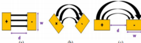
Fig. 2. Electric field lines of the IDC evaluated from the (a) parallel plate electrode to the (b) intermediate shape, resulting in (c) coplanar interdigitated electrode [10]
