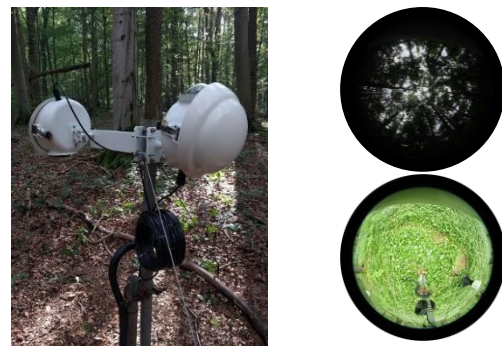
Figure 1: Automated DHP system deployed at Hainich National Park, Germany (left) and example upwards- (top right) and downwards- (bottom right) facing images.
