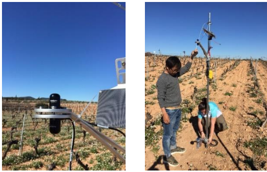
Figure 2: Wireless quantum sensor network deployed at the Valencia Anchor Station, Spain.
