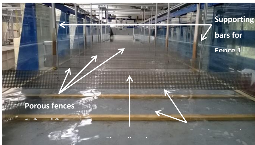
Figure 4. Porous fences positioned in the flume with row spacing, l_f=7l_z . Bed roughness positioned on the flume bed. Flume outlet with raised weir shown at the far end. Porous fences held in position using 2 thin vertical supporting bars.
